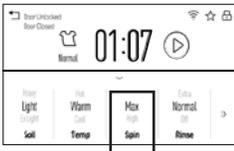
Changing the **Spin** setting changes the final spin speed of the cycles. Always follow the garment manufacturer's care label when changing the **Spin** setting.
