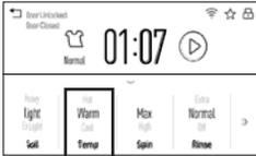
Adjust to select the proper water temperature for the wash cycle. The rinse water is always cold to help reduce energy usage and reduce setting of stains and wrinkles.
