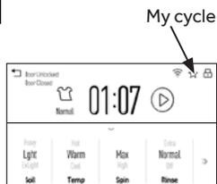
Set up your favorite combination of settings for each cycle and save them here for one touch recall. These custom settings can be set while a cycle is in progress.
