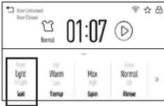
Changing the **Soil** level increases or decreases the wash time to remove different amounts of soil. To change the **Soil** level, locate the **Soil** level section on the cycle screen and scroll up or down until you have reached the desired setting. You can choose between Extra Light, Light, Normal, Heavy or Extra Heavy soil.
