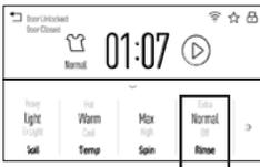
Changing **Rinse** will change the number of rinses the cycle will use. To change the rinse option, locate the Rinse section on the cycle screen and scroll up or down until you have reached the desired setting. You can choose between Normal, Extra and no rinse.
