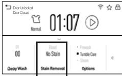
The Stain Removal guide is pre-programmed with the ideal wash and rinse settings to tackle five common stains. To use this feature, select the desired wash cycle and locate the **Stain Removal** guide menu and select the stain you want to remove. Next, press **Start**.
